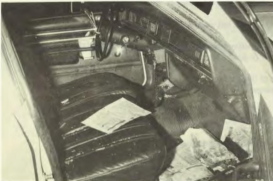
This vehicle struck a fixed object and rolled over. The extensive damage indicates the possibility of serious personal injury. However, note that the driver and passenger areas are still intact.
